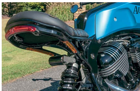
ABOVE: Neatly designed and arranged, the tail light and indicators are fitted into the subframe
